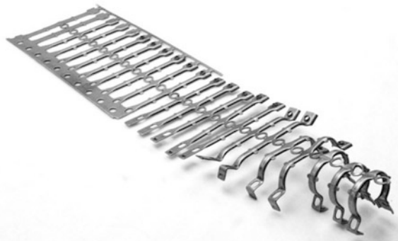
Fig. 14.7 Forming process of workpiece in progressive die ( http://www.gestiondecompras.com )
