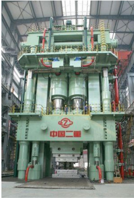
Fig. 14.4 Large die forging machine made in China
