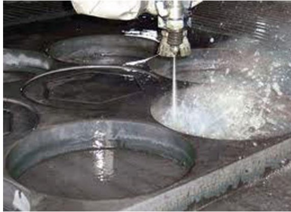
Fig. 12.13 Thick steel plate cut with water jet ( www.allsetengineering.com )
